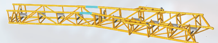
Stinger Member Structural Checks
